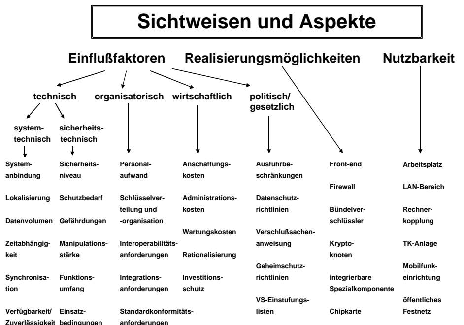
Figure: Perspectives and aspects in the selection of cryptographic procedures and components
